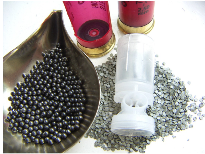
24gram Steel shot cartridge components
