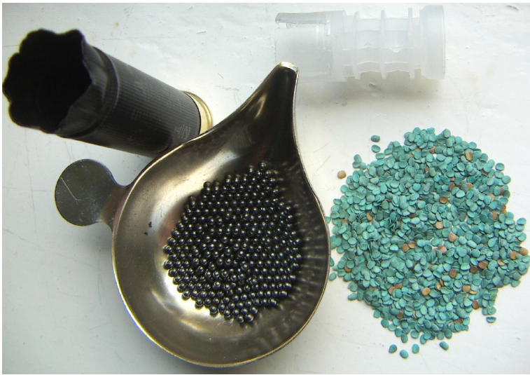
21gram Lead shot cartridge components
