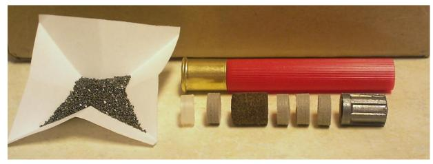
Built up Gas Seal, Nitro Card, & Cushion Wad Load Method:
