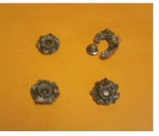
0.8 inches diameter thus nearly doubling in frontal area. Weight retention for the three test slugs that held together was nearly 100% and the one that broke apart still maintained over 90% of it's weight in the two main chunks which were found together in the orientation and spacing that I lined up for the photo. The smaller nose chunk penetrated a half newspaper layer deeper then the main ring.
