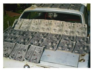
then buried itself in the first few layers of the second bunk of wet newspaper. The other three slugs were found in the last layer of the first bunk bulging out the backside of the bunk.
