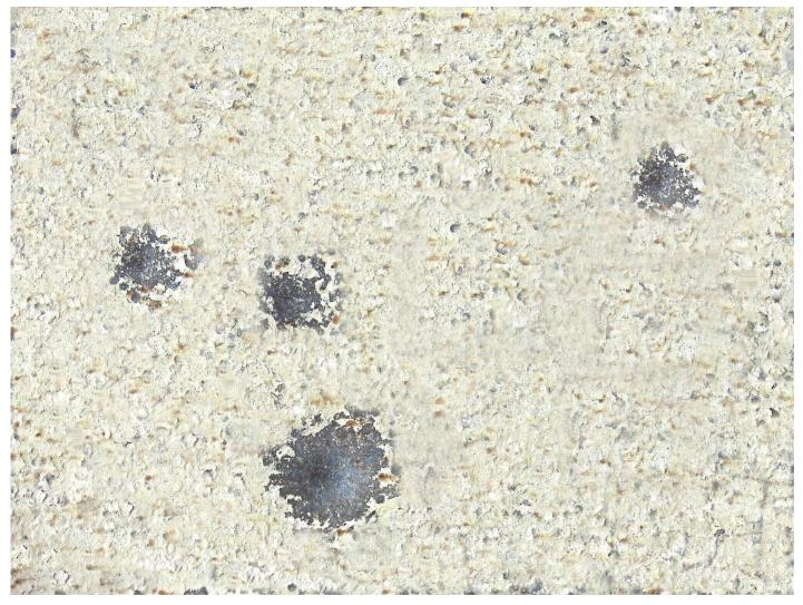
The impact on the pattern plate of the entire shot charge welded into four clumps of 'balled' shot (one larger and three smaller) caused by hot powder gases leaking past the wad, when a shorter fibre wadded 2¾ inch (70mm) cartridge was fired in a 3 inch (76mm) chamber.
