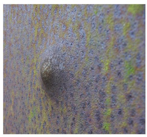
Above both left (front) and right (rear): The main 'balled' part of the charge seriously damaged the pattern plate, nearly breaking through it completely!
