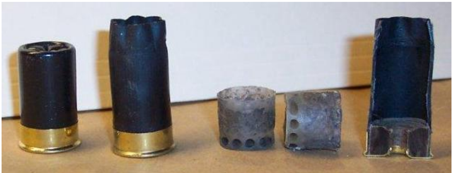
View of loaded shell, fired shell, two neat little plastic mini-wads, and cutaway showing well made three piece design with separate base wad.
