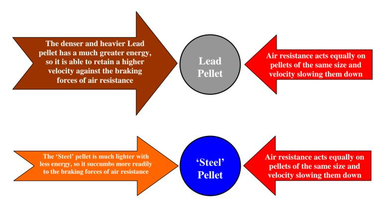
It must be appreciated that the resistance of the air to a shot pellets' flight through it is considerable. It can perhaps be compared to wading through water; a much larger effort is needed to do it more quickly.
