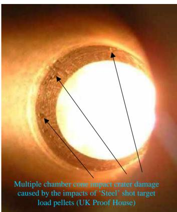
It must be appreciated that the 'Steel' pellets are very much harder than lead, needing mandatory protection of the gun's bores from any contact with them. If contact is made, this can and does, cause scoring of the barrels and impact craters at the chamber cones. Left: Evidence of this type of chamber cone damage, can be seen inflicted on a European made over and under that was only two weeks old. The bores and chokes were also badly scored.
