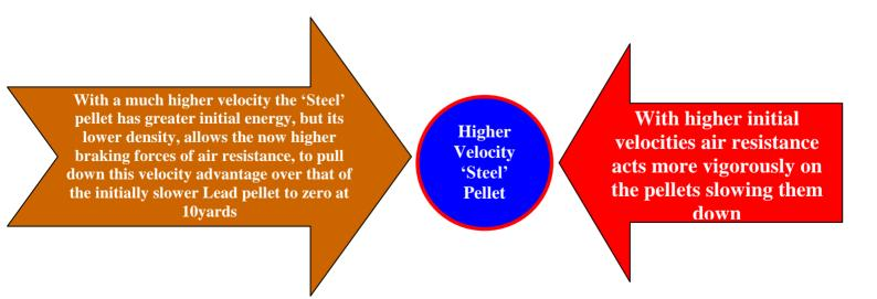
The actual effects of the lower density of the 'Steel' pellets, is shown in the retained velocity-charts.
