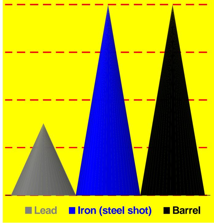
From the chart, immediately we can see that there are most definitely going to be damage issues, if there is any barrel wall contact from the 'Steel' shot (Iron) pellets.
