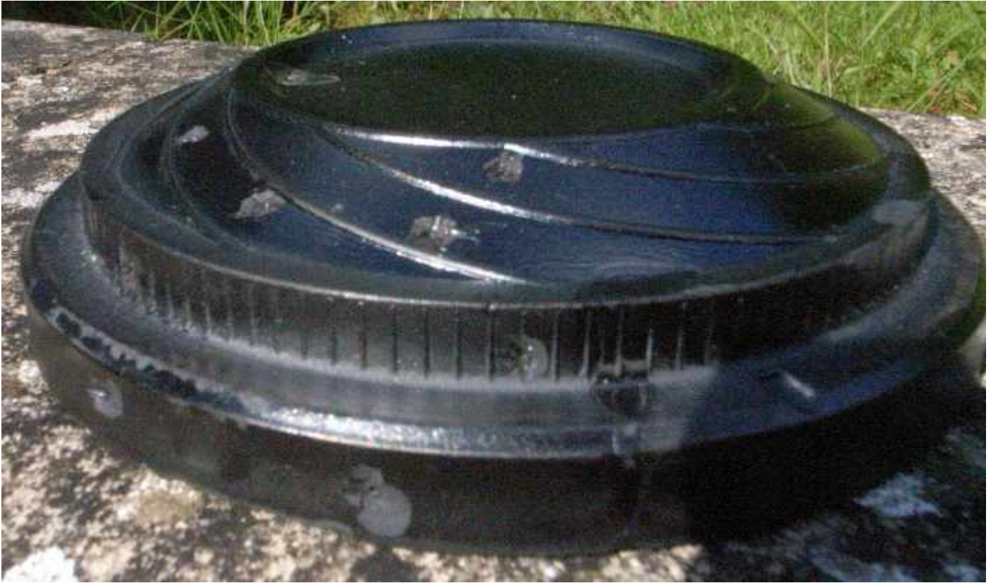
Picture 4: After receiving no less than 8 direct pellet strikes from a 'Steel' target load, (all of which ricocheted off of it), this clay pigeon flew on intact and didn't even break when it landed on the ground. The steel pellets lacked the necessary individual momentum required to penetrate the structure of the clay pigeon and break it.
