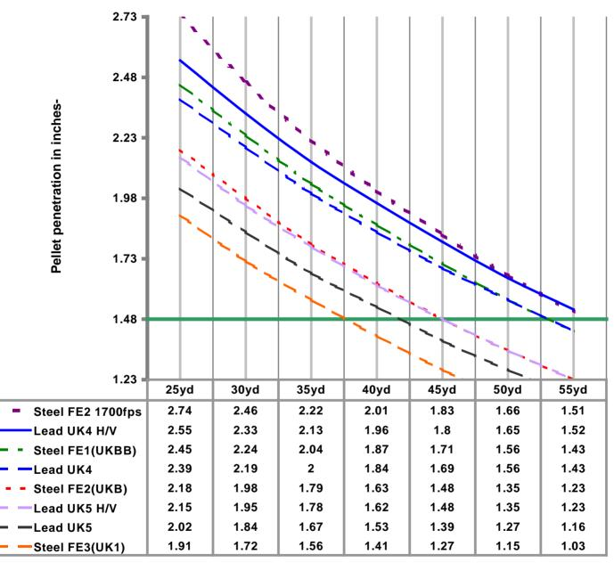
Steel pellet penetration comparison with UK lead numbers 4 & 5 shot
