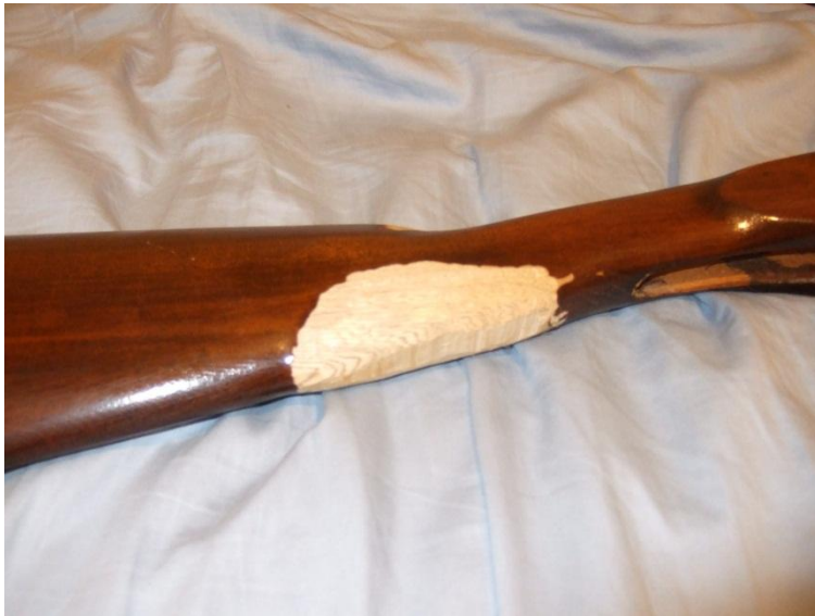
The stock right after I cut off the POW grip and carved off some of the excess wood.
