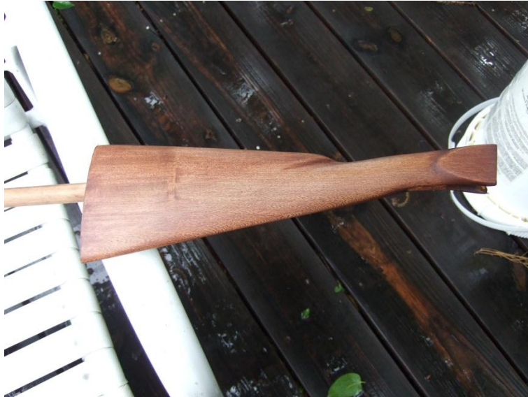
The stock after sanding with the first coat of stain applied.
